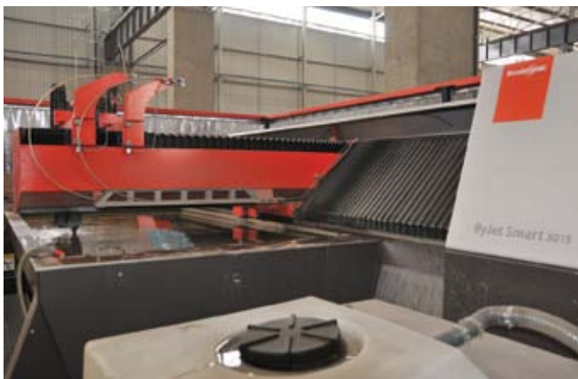
Certain clients need waterjet cutting services and Lasercraft has a Bystronic Byjet Smart 3015 to carry out these operations
