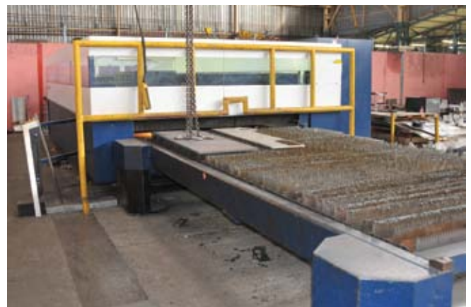
AAA Laser has a Trumf TruLaser 3040 CNC laser cutting machine with a working range of (XYZ) 4000 x 2000 x 115 mm and maximum cutting thickness of mild steel 20 mm, stainless steel 20 mm and aluminium 10 mm which was supplied by Retecon Machine Tools
