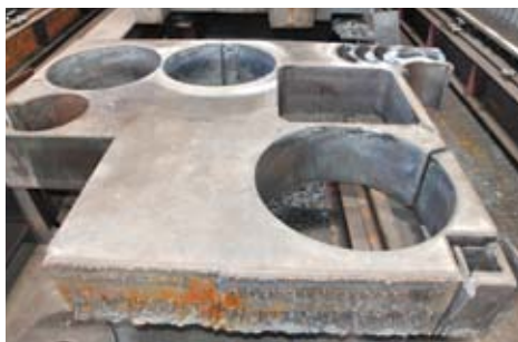
The MultiTherm CNC oxyfuel machine comes equipped with Messer ALFA gas cutting torches that have fully integrated height sensing, this not only maintains the optimum cutting height but also ensures consistent cut quality
