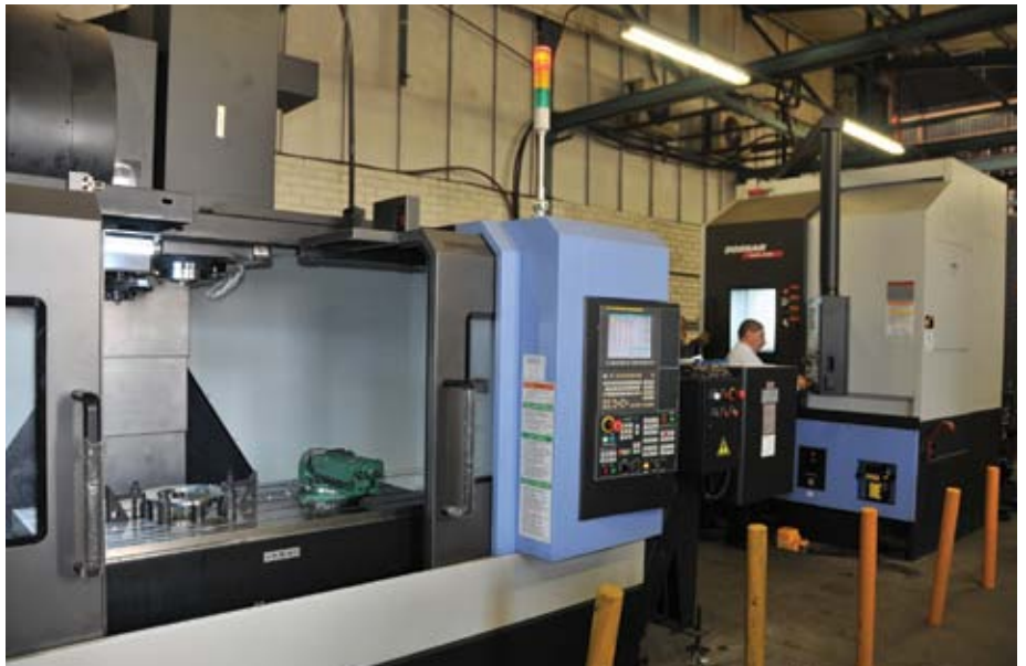
In March AAA Laser installed a Doosan DNM 650 VMC CNC vertical machining centre and a Doosan Puma V550 CNC vertical turning centre, both supplied by Puma Machine Tools
