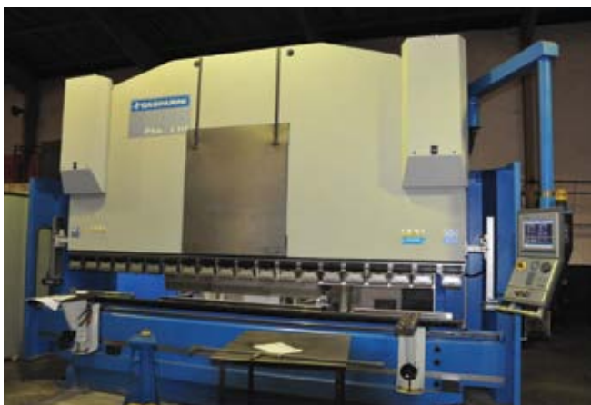
The new Gasparini PSG 330 press brake, which has a bending force of 330 ton over a four metre width, was supplied by Talmac Machine Tools
