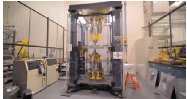
Ford Freeform Fabrication Technology uses an embossing technique similar to 3D printing
