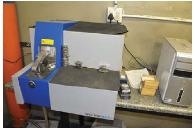
The Spectro SpectroMax spectrometer determines all of the elements used in the cast metal industry, including trace analysis of carbon, phosphorous, sulfur and nitrogen
