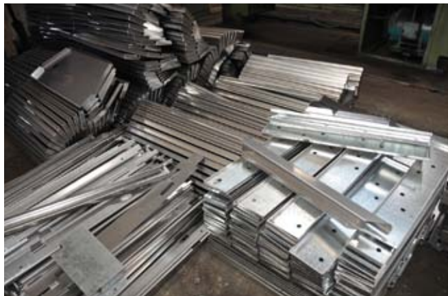
Components that have been bent on the Trumpf TruBend 3120 CNC press brake
