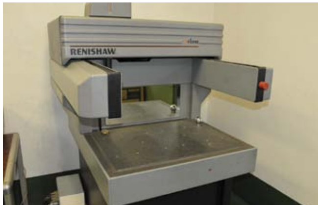
The Renishaw Cyclone contact scanner provides the company the opportunity to do direct CAD output for reverse engineering, CAM output to machine components and a host of measuring and inspection capabilities
