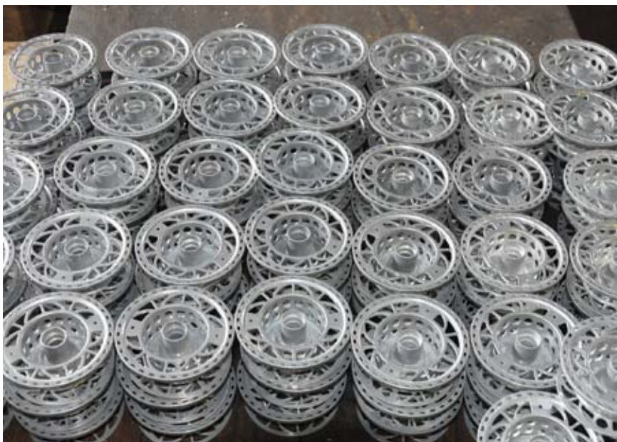
The body of the reels are machined from aluminium solid
