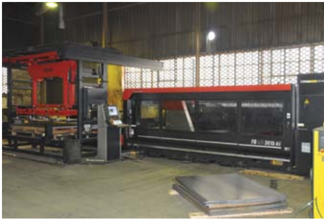
Larcol Pressings has an Amada FOM2 3015 NT laser, which represents the third generation of Amada's proven FO series that was introduced in 1999
