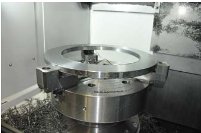
A component being machined on the Doosan Puma V550 CNC vertical turning centre
