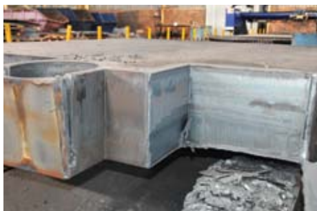
The MultiTherm CNC oxyfuel machine has the capability of cutting mild and low alloy steels up to 300mm thick
