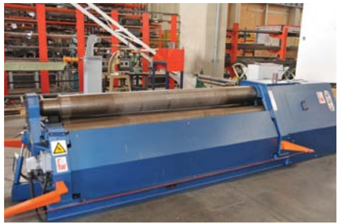
Lasercraft has a Faccin three roll double pinch plate bending machine, which is ideal for light materials and low volumes. The machine was supplied by Talmac Machine Tools
