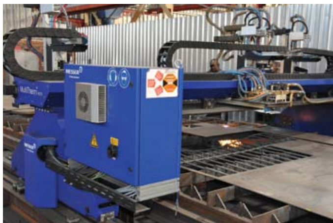
Messer Cutting Systems supplied a MultiTherm CNC oxyfuel machine with four gas heads in 2013
