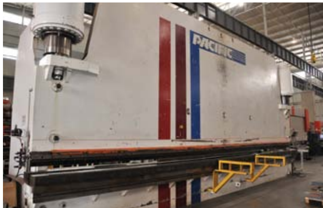
Lasercraft have incorporated a Pacific CNC I 250 ton hydraulic press brake into their equipment register. The CNC press brake has a 10 metre bed, weighs in at 160 tons, has a 6-axis backgauge, hydraulic upper tool clamping and a remote laser alignment system
