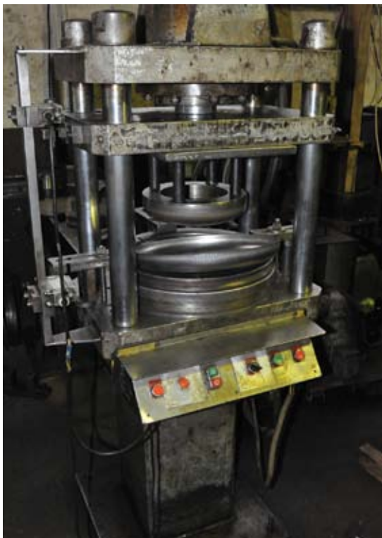
Larcol Pressings has a press and offers dished end pressings as a service
