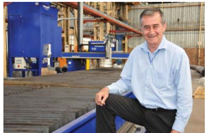
Dimitri Anastasiu, owner of AAA Laser, stands in front of the Messer MultiTherm CNC plasma machine fitted with a single Kjellberg Hi-Focus 440i plasma cutting unit, that was installed earlier this year
