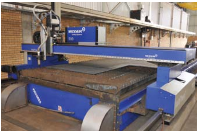
The Messer Multitherm plasma cutter
