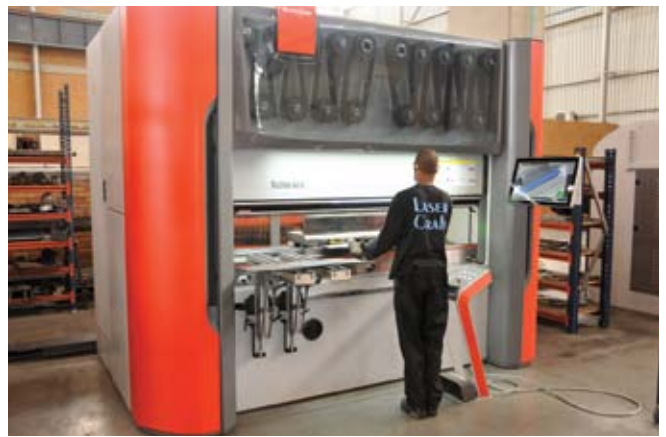
One of the more recent machines that Lasercraft has purchased is a Bystronic Xcite 80 E CNC press brake
