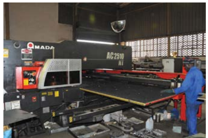
On the punching side Larcol Pressings has an Amada AC2510NT Turret Punch
