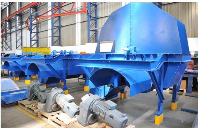
All of Malvern Engineering's components are assembled and tested on site at their fabrication facility before being freighted to customers
