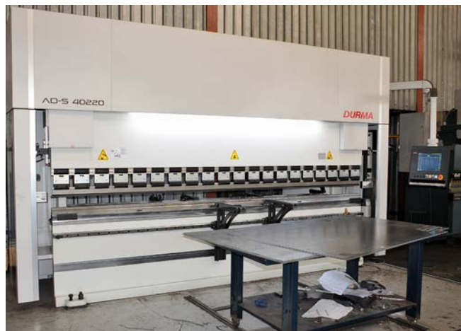
The new Durma AD Servo 40220 hydraulic press brake that has a bending length of 4 020mm and a bending force of 220 tons installed by Spectrum Machine Tools Africa
