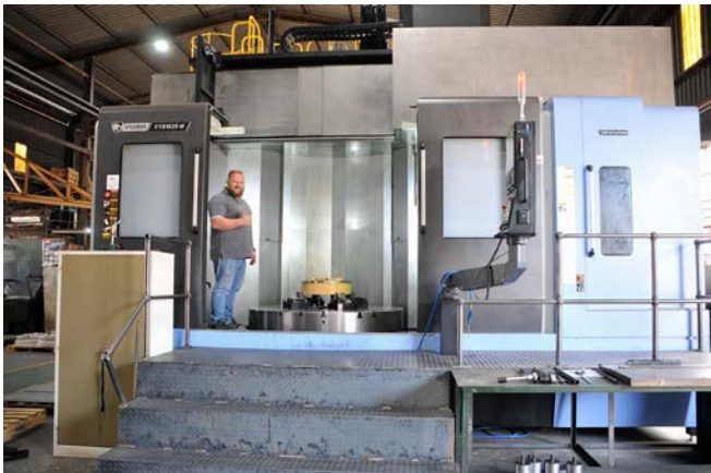
Gauteng-based Simmer Engineering have recently installed a new, large-capacity DN Solutions Puma VTR1620M ram type vertical borer that positions the company in the large component machining category. The machine was supplied by the Retecon Group company Puma Machine Tools. Machine shop manager Rudolph van Tonder gives an idea of the size of the machine
