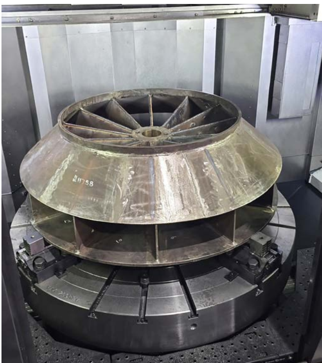
New machine, new client, new work. This component – a blower fan that weighs 950kg and has a diameter of 1 950mm – is part of a new order that Simmer Engineering has recently acquired
