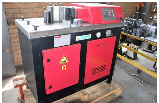
Staluform make use of a Nargesa machine for bracket manufacture
