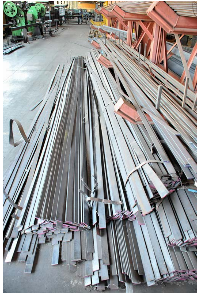
“We are processing in the region of about 200 tons of material each month. This does not include the 47mm x 5mm flat bar that we import. The bar is generally only used in the forming industry for creating structural type components like braces, support straps, clamps, brackets and custom components but is used in other areas of fabrication.”
