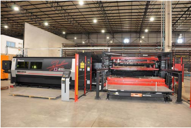
Hitech-Gregfor have recently installed an Amada ENSIS 3015 6kW fiber laser that has been paired with an Amada MPL 3015 C manipulator that incorporates a shuttle table function
