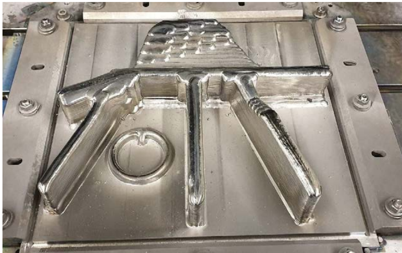
w-DED, on the other hand, allows Airbus to move from printing small components to creating large, structural titanium parts up to seven metres long
