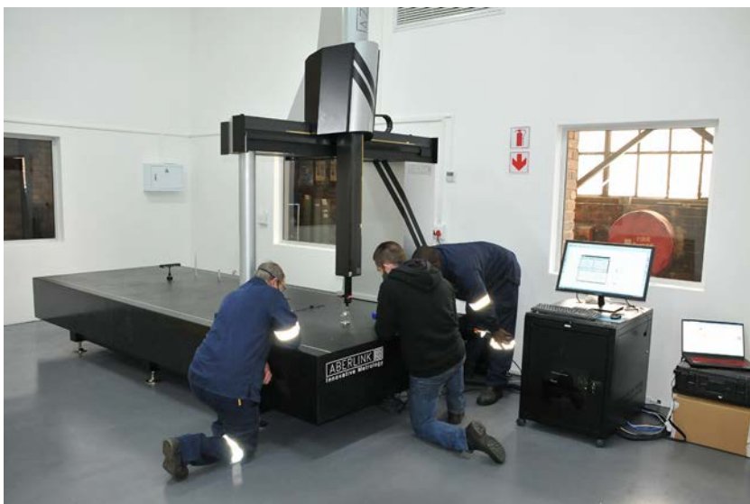
Simmer Engineering invested in an Aberlink Azimuth CNC CMM that was installed in a purpose-built temperature-controlled room so as to offer clients a CMM service which is being called for regularly these days
