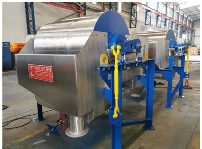
Malvern Engineering's wet drum magnetic separators are high-efficiency magnetic separation systems that ensure effective recovery of magnetic materials from slurries. Image courtesy of Malvern Engineering
