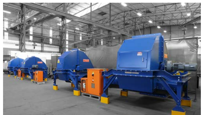
Sampling systems form another technical segment of Malvern Engineering's fabrication abilities. They fabricate cross belt samplers, rotary sample dividers and variable split sample dividers. Image courtesy of Malvern Engineering
