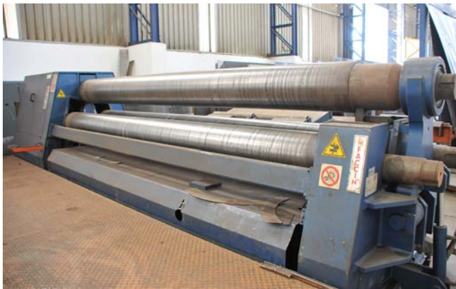
Fabrication takes place in meticulous order from raw material to finished components – with shot blasting and painting all taking place at Malvern Engineering's warehouse. Pictured is a Faccin 3-plate roller used for fabrication of rolled components
