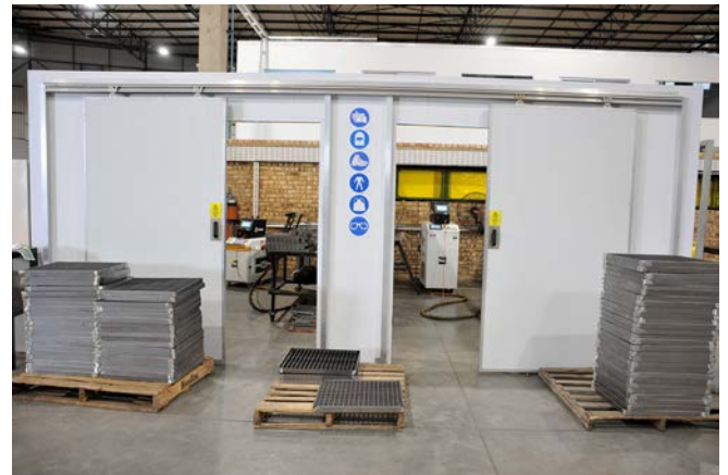
“We have also decided to invest in five hand-held laser welding systems from Hugong HGLW and supplied by TRM Supplies because of the potential it offers in our shop environment that we operate in. Manual fiber laser welding will never replace the traditional MIG and TIG welding processes. Each individual unit has its own closed enclosure so there are no safety issues.”
