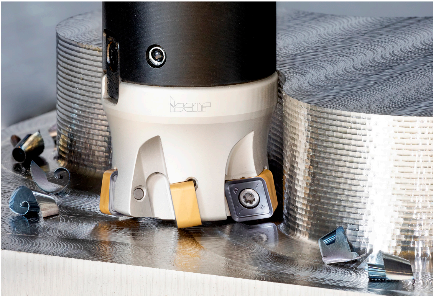
Fig. 3 Iscar's FAST FEED technology is particularly effective in pocket milling and roughing operations where cycle time reduction is critical
