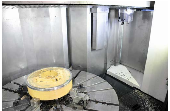
The machine has X axis travel of 2 220mm and a Y axis travel of 1 200mm, which gives you a maximum swing diameter of 2 100mm, a maximum turning diameter of 2 000mm and a workpiece height of 1 800mm
