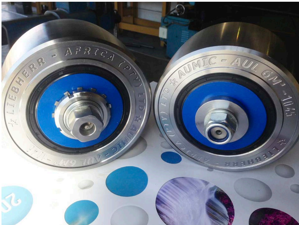
“One thing we have been quite well-known for over the years is our roller engineering. I designed and engineered a fully sealed roller that targets the needs of the cement truck industry. We decided to call our roller the S-2 roller and I redesigned it to have bigger bearings but more importantly to be a fully sealed unit.”
