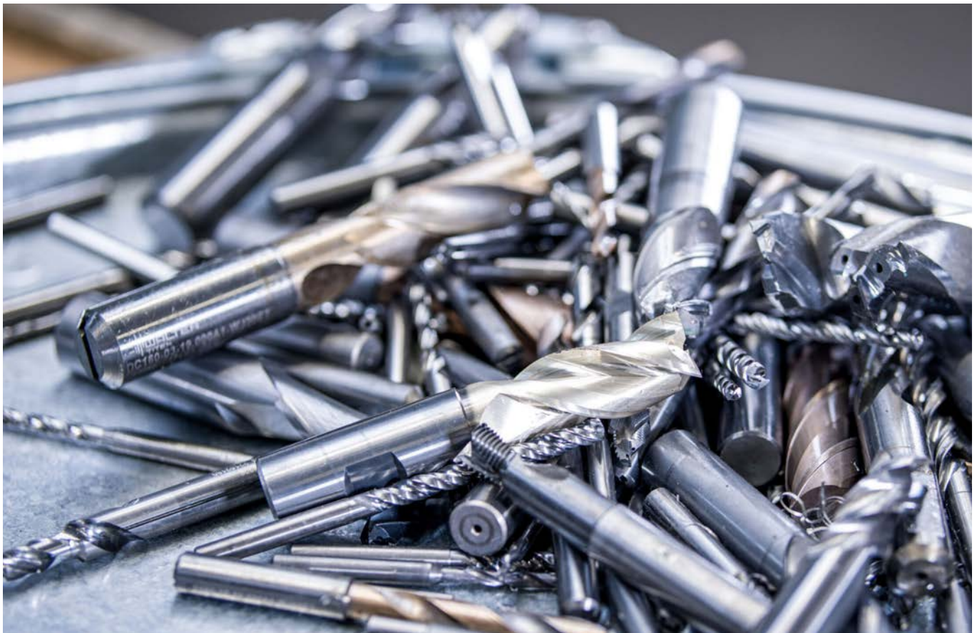
Gühring purchases worn tools and other carbide scrap, feeds it into the recycling process and extracts valuable secondary raw materials from it, which are used to manufacture new, high-performance tools
