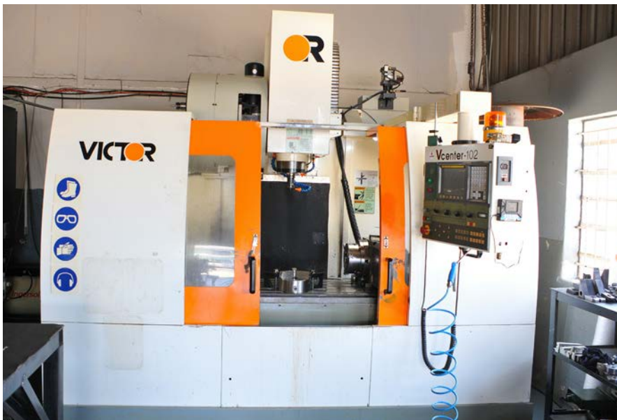
Aumic Engineering's Victor Vcenter 102 vertical machining center is equipped with a 4th axis rotary table – the rotary table gives Aumic Engineering an ability to machine complex and intricate components
